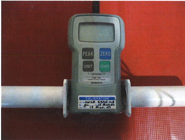
Shimpo FGE-100 digital push-pull force gauge. Note there are several models of push-pull force gauges that can be used.
