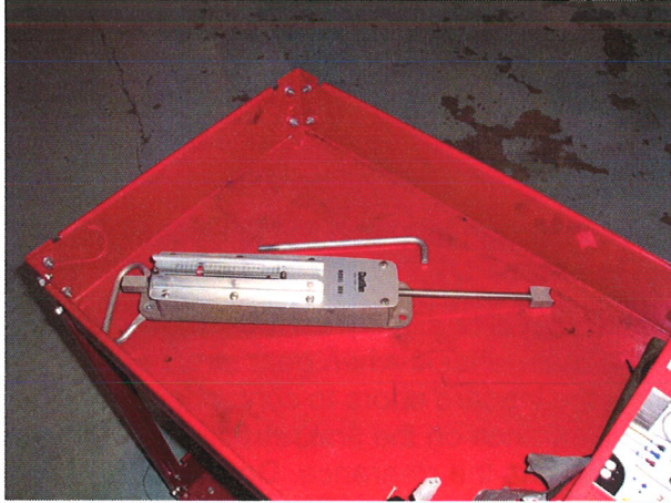
Chatillon Model 80D mechanical push-pull force gauge. This commonly used gauge is no longer in production.
