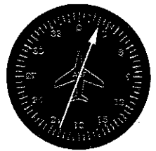
DIRECTION INDICATOR Indicates the bearing of a station in degrees of azimuth relative to the fore-and-aft line of the aircraft.
