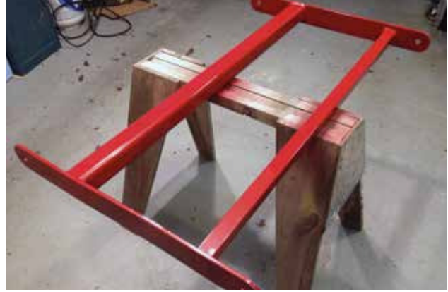
The lifting arm welded and painted. I found that painting as I went was a small morale boost and allowed me to gauge my progress.
