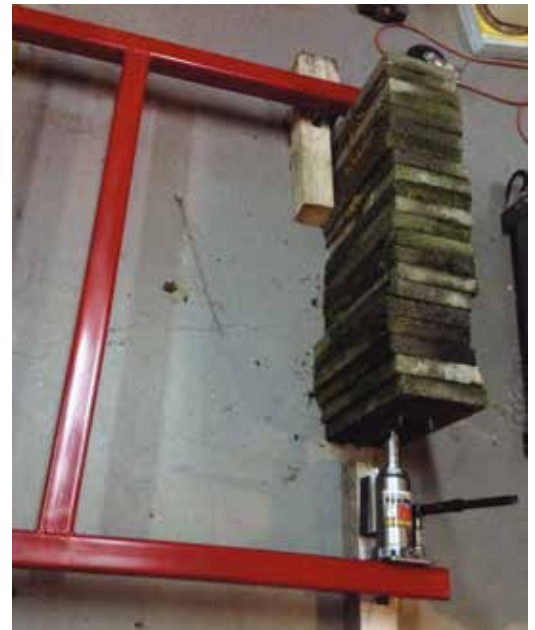
Welding causes contraction. To make room for the lifting arms between the lower frame arms, I had to move them out a half inch. An 8-ton bottle jack was perfect for the job.
