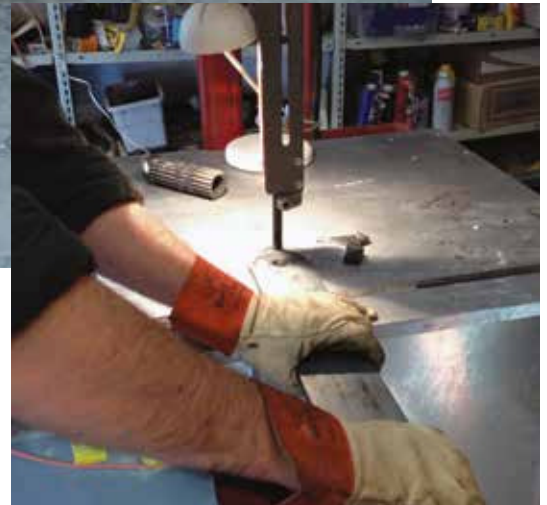
A bimetallic hacksaw blade on an old band saw makes cutting the 3/8" bar or 2-1/2" tube easy.
