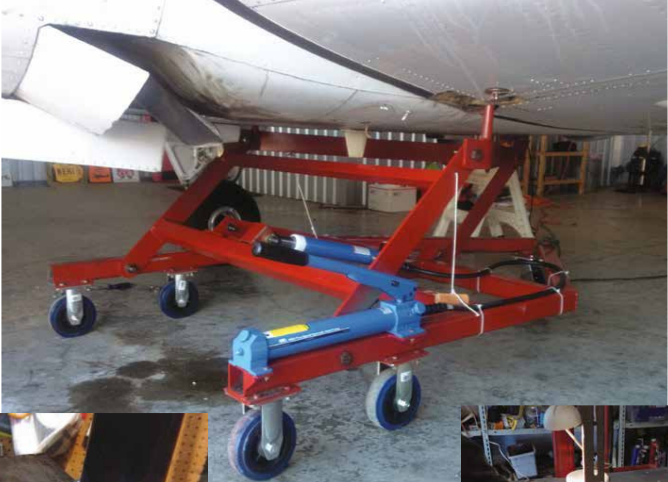
The jack worked flawlessly. Raised and secured, we were able to swing the gear with confidence.
