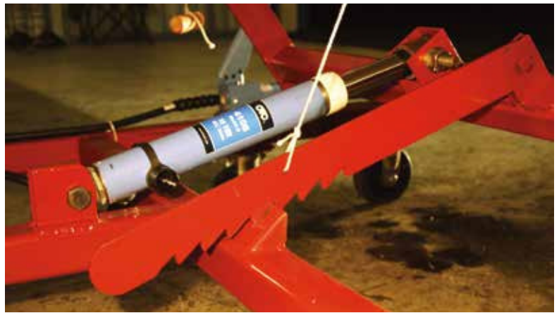
The plans called for a safety rod – I thought of a notched bar of 3/8" steel that easily holds the weight of an aircraft.
