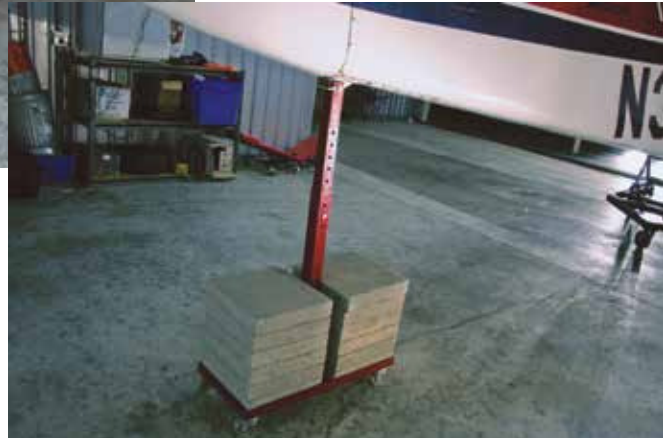
It's possible to lift and move the aircraft with the jack alone, but in order to work on the aircraft, especially the aft fuselage, a tail stand makes things much more stable and secure.
