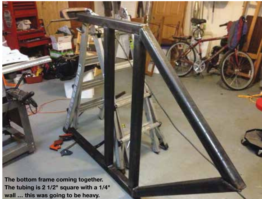
Welding causes contraction. To make room for the lifting arms between the lower frame arms, I had to move them out a half inch. An 8-ton bottle jack was perfect for the job.
