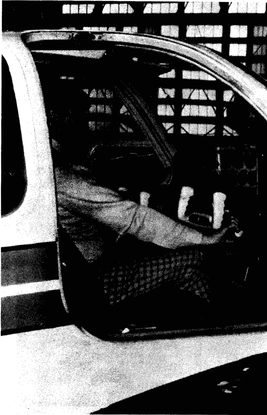
Figure 7.—Pilot reaching underneath the control wheel bar to locate obscured landing gear control switch.
