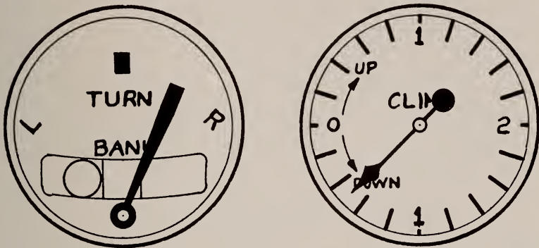
Fig. 15—This Illustration Indicates a Turn, Skidding Out, and Descending.
