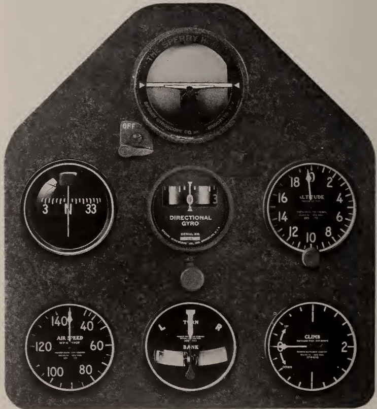
Fig. 3—Combination arrangement of Sperry and Turn Indicator Group.
