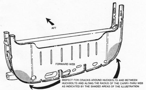
INSPECTION FOR CRACKS IN THE WING FORWARD SPAR CARRY-THRU
