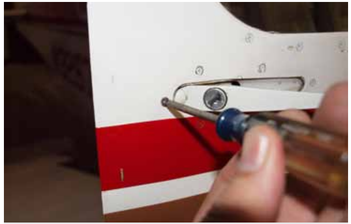
10. Tail of old spring is sandwiched between door skin and door handle mount casting. The rear screw holds it in place. Loosen or remove the screw to remove old spring tail.
