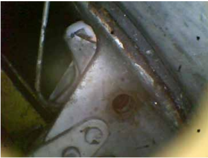
7. Upward view after clevis pin was removed. Tail of old spring is visible at left. Also at left are the two green “flat plates”, mentioned in steps 13 and 15b.
