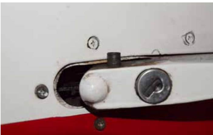
9. Bushing after being pulled upward a bit. You can remove main part of old spring with forceps.
