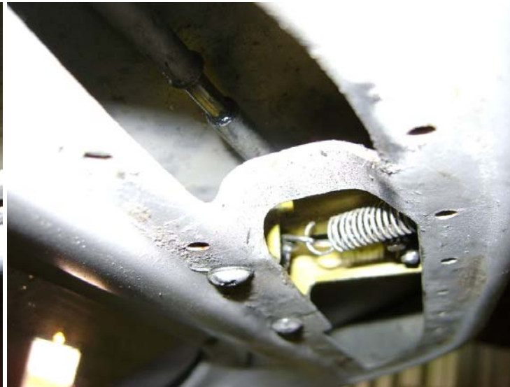
Upper Door Latch mounting looking aft
