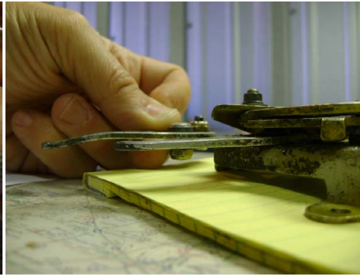
Notice the severely bent hook arm. This is pretty FUBAR!
