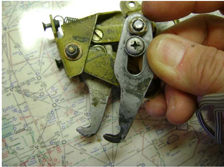
Notice the huge amount of wear in the "hook" on the right.
