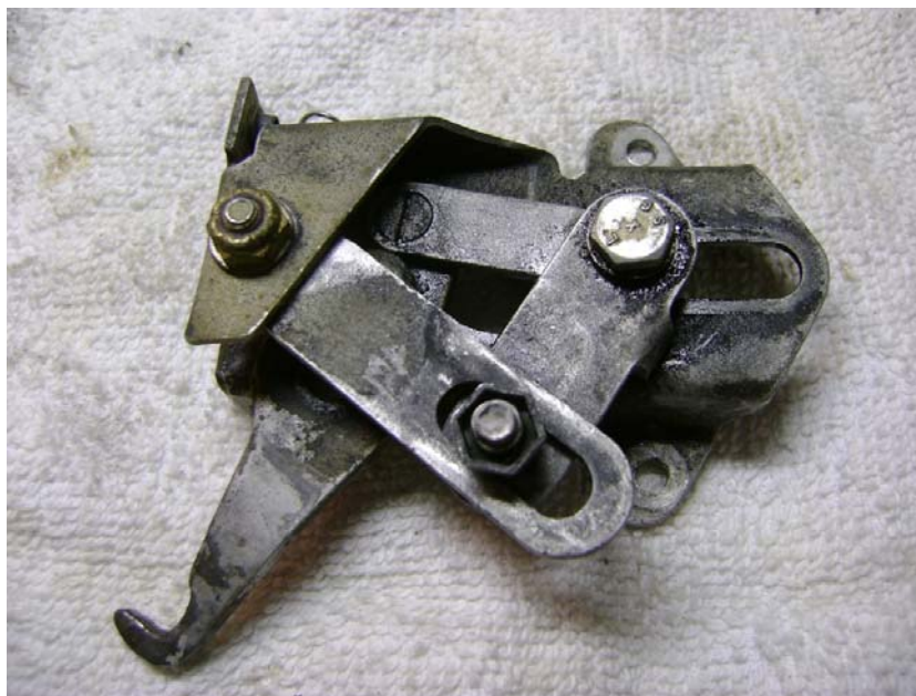
My Worn & Bent Upper Door Latch
