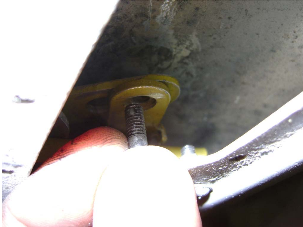
Bolt through latch arms connects to push-pull tube, nut attaches on top.
