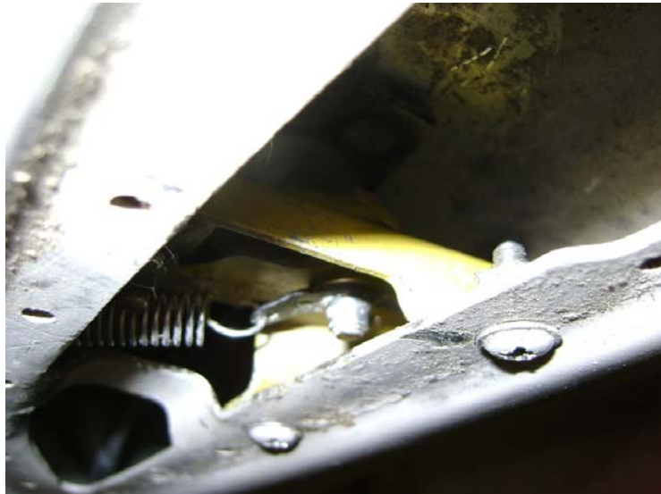
Upper Door Latch mounting zone from underneath
