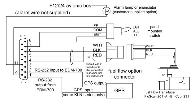
The fuel flow connector is attached to the instrument by a short cable. The plug should be pre-wired with a harness. Fuel flow option connector pin assignments are as follows:
