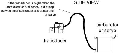
**elbow joint immediately prior to the input port of the fuel flow transducer.** There should be six inches of straight flow immediately before the transducer input port.
