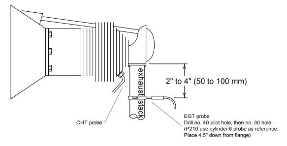
Insert the probe in the exhaust stack hole such that the tip of the probe is in the center of the exhaust stream. Tighten the stainless steel clamp and torque to 45 in/Lbs. Cut off excess strap close to the screw. The probe warranty is void if the probe is mounted in any type of a slip-joint.
