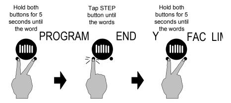
Tap the STEP button to advance to the next item in the list. Tap the LF button to select alternate values of that item. Hold the LF button to rapidly back up. Prompts listed in the first column are displayed for only two seconds.
