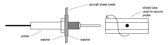
The outside aluminum shield tube is used to both hold the probe in place, protect it from damage, and shield it from radiated heat. OAT will be shown in the digital part of the display as, for example, 75 OAT. When testing the OAT, shield the sensor from direct sunlight and engine heat, while the engine is operating.
