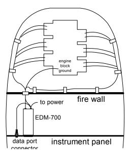
probe, sensor and transducer leads to a convenient location on the engine approximately 8 to 12 inches from the probe, sensor or transducer, being sure there is sufficient slack to absorb engine torque. It is essential in routing the probe, sensor or transducer wire that this wire not be allowed to touch metal parts of the airframe or engine since abrasion will destroy the wire.
