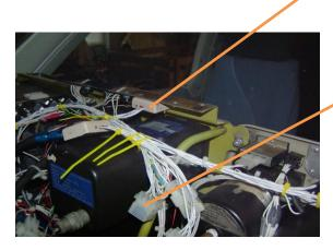
Fuel PC Board located under the glare shield. NO NEED to remove it for the test
