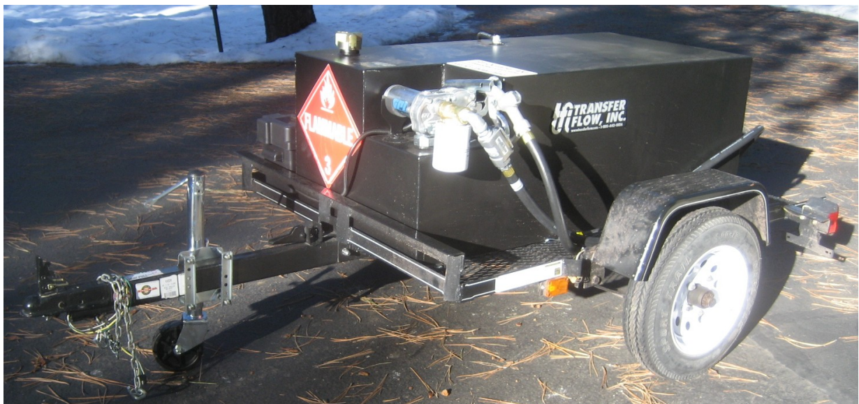
Tank Bolted Down, Filter, Hose, Nozzle, Meter Installed
