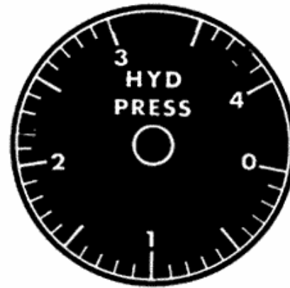
HYDRAULIC SYSTEM PRESSURE GAGES (A AND B-L AND R)
