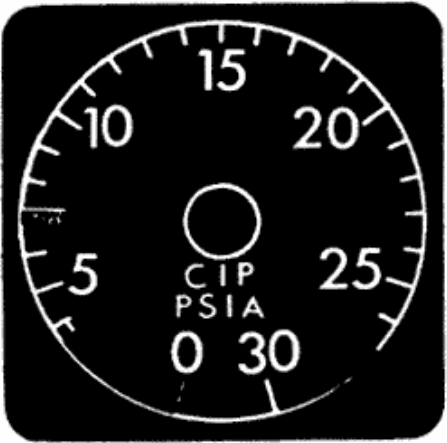
COMPRESSOR INLET PRESSURE GAGE 7 psi-Minimum for airstart
