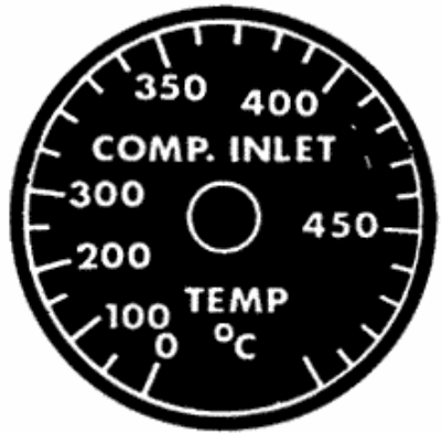
COMPRESSOR INLET TEMPERATURE GAGE
