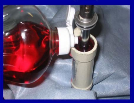
Center fixed piston is near bottom end of barrel. An old soap bottle makes filling the barrel with 5606 easier. Fill to very top from clevis end. Eliminate bubbles.
