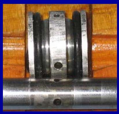
Shaft has two large holes for fixation pin and one small fluid transfer hole.
