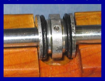
Slide piston on shaft. Line up holes.
