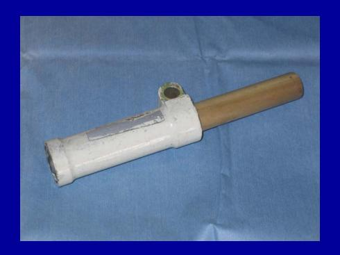
The opposite end cap and scraper ring may need to be pushed out in the opposite direction using the wooden dowel.
