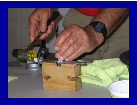
Tap out pin holding center piston with punch.
