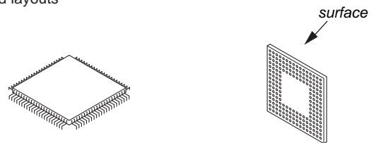
Lead layout of conventional IC
