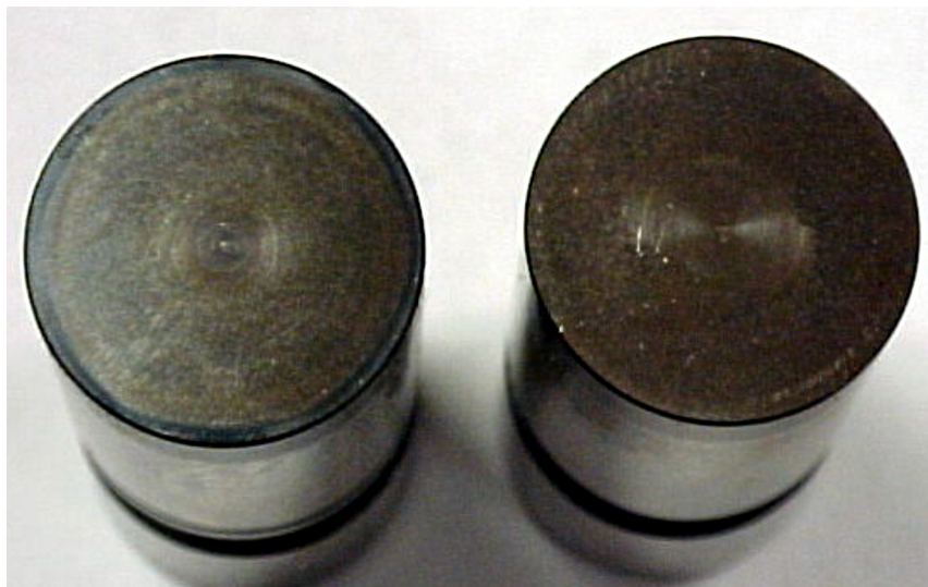
Figure 6-106.3. Typical Lifter Faces in Service
