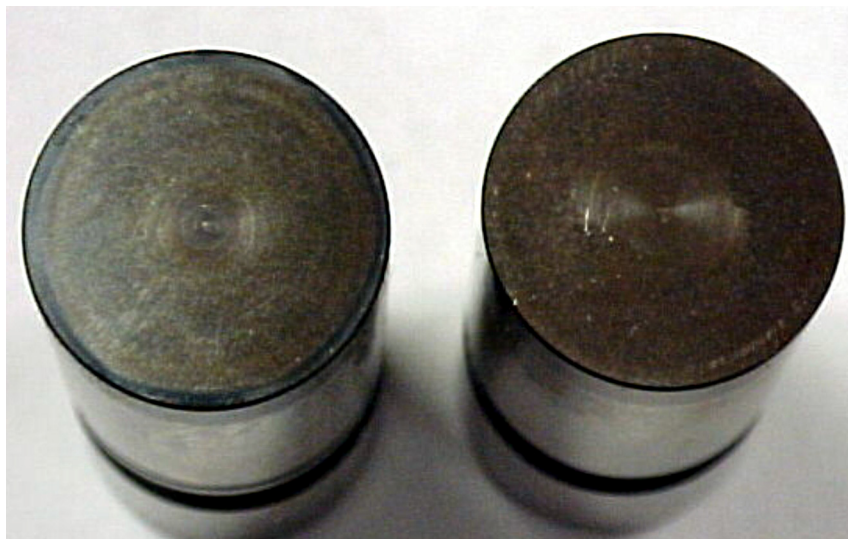
Figure 6-106.3. Typical Lifter Faces in Service
