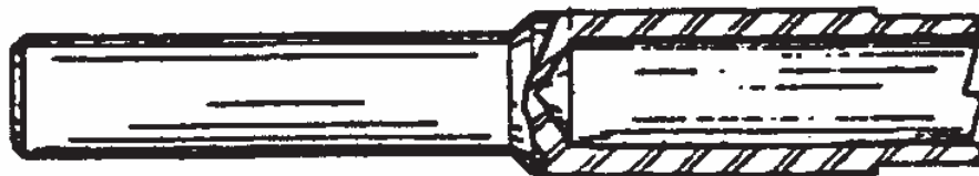
Figure 2-24. Rosan® Stud Removal Tool
