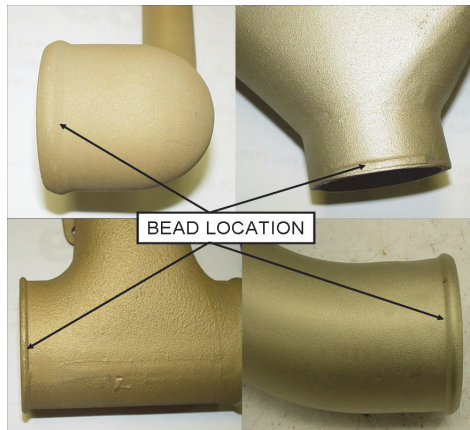
Figure 6-90. Induction Tube Bead Location
