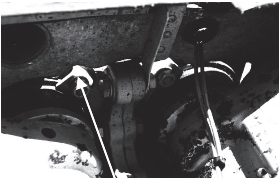
Figure 6-79. Aft and Side Baffles with Air Gaps
