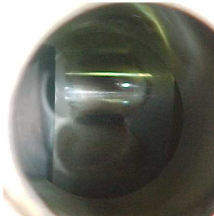
Figure 6-106.9. Cam Lobe Viewed Through Lifter Bore
