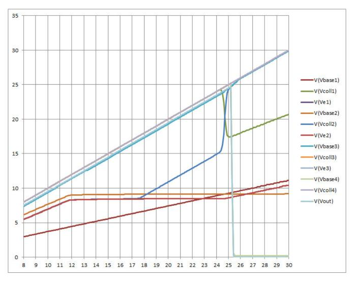
Overvoltage circuit plot of the transistor base voltages and SCR gate voltage. Q1 and Q2 in the plots are Q5 and Q6, respectively, in the schematic. As with the regulator circuit, the trim pot changes the slope of the blue voltage line, and therefore changes the intersection point of the two voltages.
